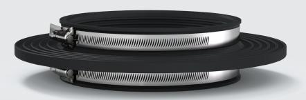
Fernco Puddle Flanges are used to seal around the outside of pipes that are required to pass through concrete structures, such as tanks, manhole chambers, shafts, floor slabs and basements and are installed during construction.
