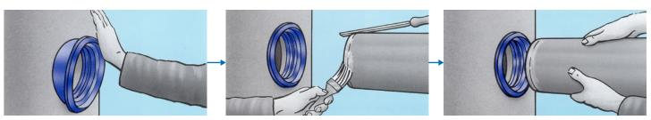
Press the Wall Seal seal into the hole. Do NOT use lubricant.
