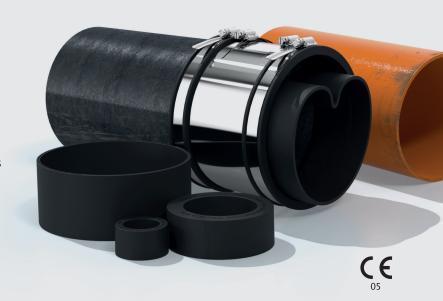
Bushes are used as an additional component part of either Shear Banded Couplings or Lateral Connection Saddles. The purpose of a bush is to increase the outside diameter of a pipe to be connected if the pipe is too small for the coupling being used or the saddle being used.
