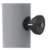
3. Insert the Access Point into the hole so that the curvature of the seal follows the curvature of the main pipe.
