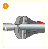
Press and hold the start button for approx. 3 seconds to trigger the pressing process. The process now runs automatically. In case of danger interruption of the pressing process is possible by pressing the emergency stop button. After resetting the the emergency stop situation, a new pressing or, if necessary, a new press process must be started.
