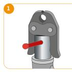
Select the pressing jaw according to the fitting and ensure clean, smooth surfaces. Insert the pressing jaw into a suitable pressing machine by opening the retaining bolt and closing it completely.
