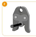
Select intermediate adapter to suit the dimension. On electronic press machines for dimensions from 40 mm to 63 mm and for conventional press machines, insert intermediate jaw ZB 203 (SANHA catalogue no. 6930) in the press machine and close the retaining bolt.
