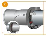
Place the press sling around the press fitting so that the bead of the fitting the bead of the fitting engages in the groove of the press sling. The press sling must fit tightly against the fitting. The marking lines on the sliding segments and the press sling must form a line. If this is not the case, the sliding segments must be made movable.
